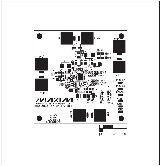
Figure 2. MAX15003 EV Kit Component Placement Guide—Component Side
