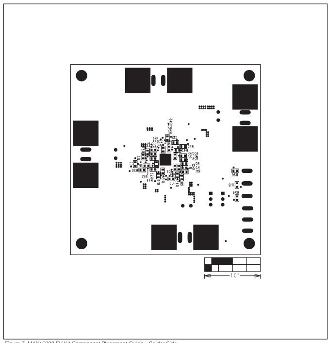
Figure 7. MAX15003 EV Kit Component Placement Guide—Solder Side
