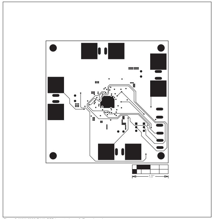
Figure 5. MAX15003 EV Kit PCB Layout—Layer 3 (Power Layer)
