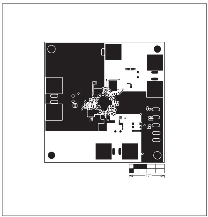
Figure 6. MAX15003 EV Kit PCB Layout—Solder Side
