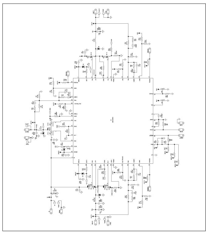
Figure 1. MAX15003 EV Kit Schematic
