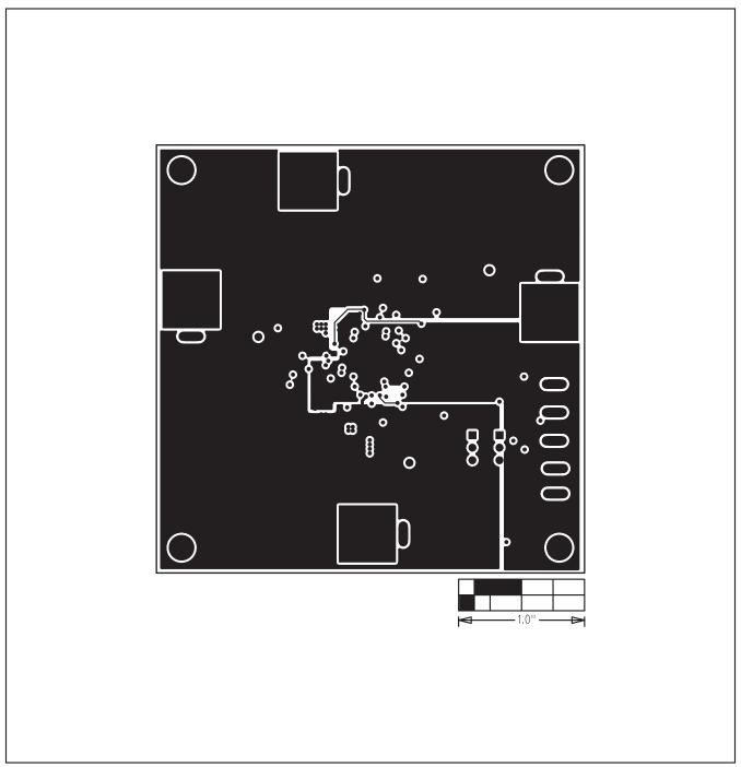
Figure 4. MAX15003 EV Kit PCB Layout—Layer 2 (Ground Layer)
