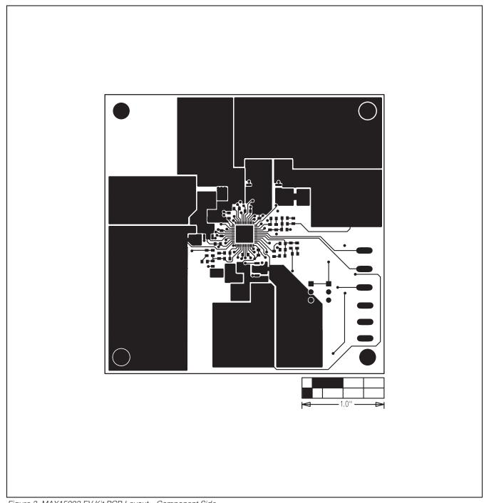
Figure 3. MAX15003 EV Kit PCB Layout—Component Side
